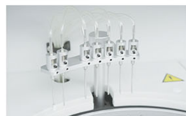
Washing Probe Independent 7-step washing system.
